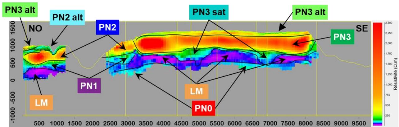
**Figure 3:** Example of an interpolated resistivity profile along the existing underground Salazie amount gallery, with geological interpretation. PN0 to PN4 represent old to recent volcanic formations.
