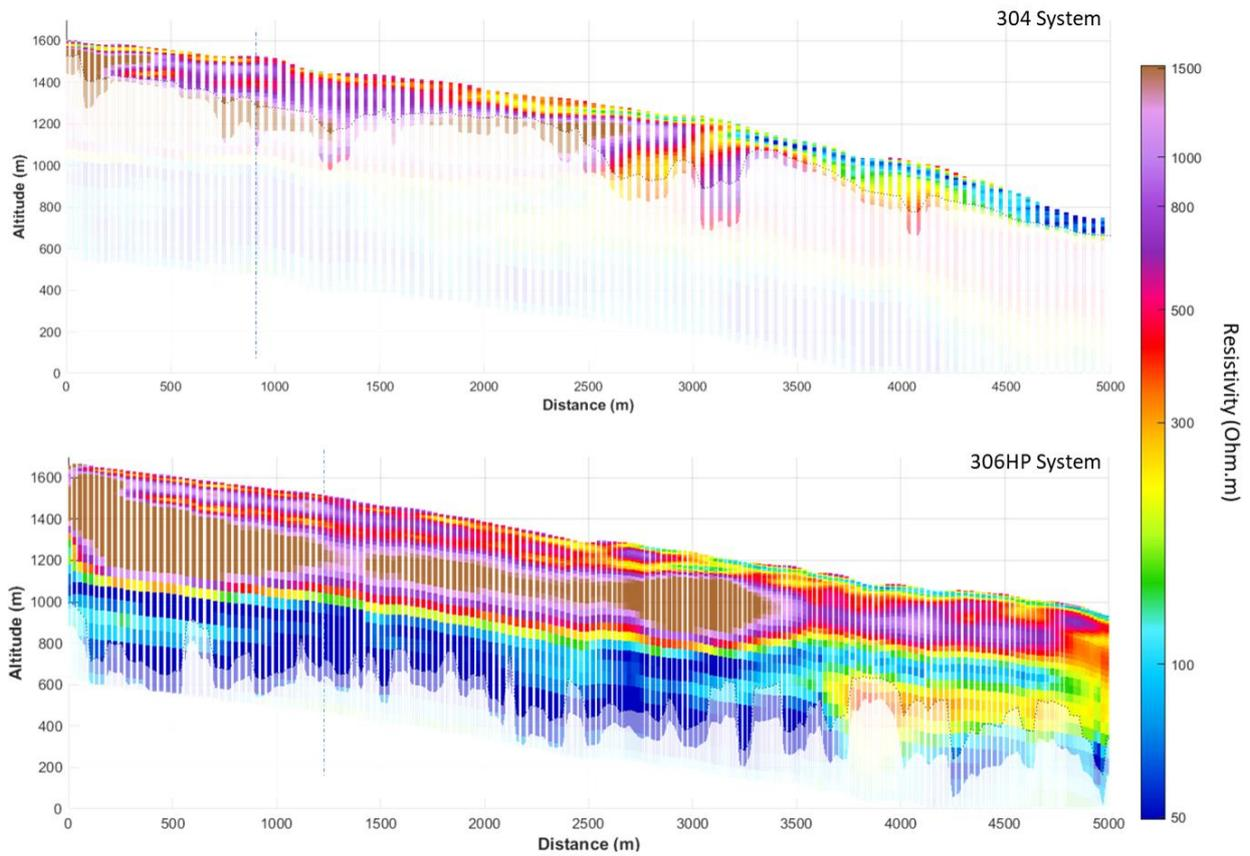
**Figure 2:** South-North resistivity profiles acquired with 304 (a) or 306HP (b) systems in the Plaine des Fougères area.
